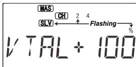
5. If the left (CH4) ruddervator moves down with up elevator stick, change its travel direction by pressing the Cursor Right key (the numeral 2 and SLV (Slave) will be flashing ng), the Active/Inhibit (Clear) key (sets 0%), then press the Data -Decrease key until you reach -50%. Otherwise, continue.
