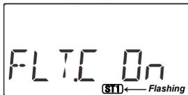
1. Get to the FLT.C screen with the Edit Up Down keys. The display will indicate "Inh" and, depending on the positions of the two controlling switches, one of the
