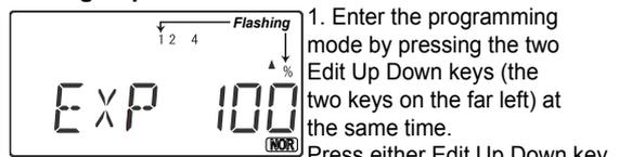
1. Enter the programming mode by pressing the two Edit Up Down keys (the two keys on the far left) at the same time.
