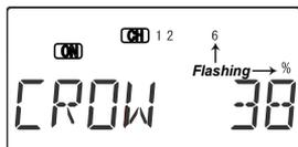
**27.** (4WNG only) Now set up the throws for the flaps as desired. Press the Cursor Right key once to get to the flap setting menu (the Numeral 6 and percentage sign will be flashing).
