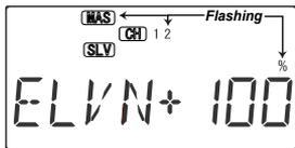
6. Press the Cursor Right key once, to get to the elevator travel setting menu. Highlighted MAS sign and Numeral 2 Will be flashing that represents elevator master
