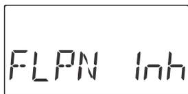
**13.** Press both Edit keys to get to the regular programming menu. The end-point adjust menu.(EPA) should appear. Press the Down arrow three times to get to the flaperon menu (FLPN). The display should show that it is inhibited (INH).
