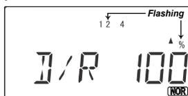
**54.** Elevator dual rate setting: press the Right Cursor key one time to get the numeral 2 to flash. Now set the elevator dual rates in the same way you set the ailerons in the previous step.
