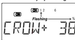
4. Next, set up the throws for the ailerons. Press the Right key two times to get to the aileron setting menu (the numeral 1 and percentage sign will be flashing in the display).
