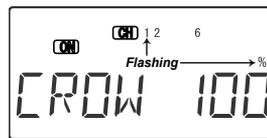
**25.** Next, set up the throws for the ailerons. Hit the Cursor Right key two times to get to the aileron setting menu (the Numeral 1 and percentage sign will be flashing).
