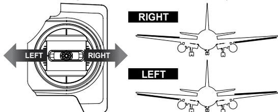
**18.** If it does not, activate the opposite direction for the CH1 aileron servo by pressing the Active/Inhibit (Clear) key. Each press switches from Reversed to Normal and
