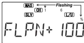
4. Press the Cursor Right key once. Highlighted MAS sign and numeral 1 will be flashing that representing right aileron master channel, and the percent indicator will blink
