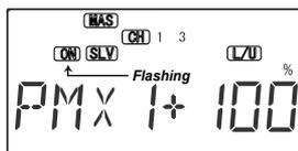
**70.** Be sure you understand how to use the CH. 7 switch to turn PMX1 on and off, since you won't want this mixing on during normal flight, only during knife-edge. Later, after you fly the model you may fine-tune the amount of elevator travel so that the pitching tendency is eliminated. You can define another mixer to handle adding aileron cor
