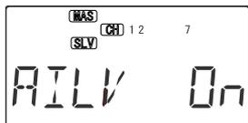
3. Press the Active/Inhibit (Clear) key to activate the Ailevator function. This will show the On indicator.
