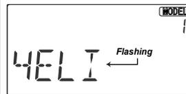
2. Press the Down arrow key. This gets you into the type select menu. The current model type will be flashing on and off. (If you're already
