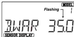
1. With the transmitter switched off, turn on your transmitter while pressing both of the two Edit keys (the two keys on the far left). The B.WAR select (B.WAR)
