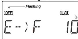
**63.** Be sure to input a mixing percentage for each side of the elevator stick motion.
