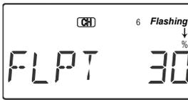
1. Use the Edit Up Down arrow keys to select the FLPT window. 2. Pressing the Data +Increase or -Decrease key to input your desired flap motion setting. The 30% default value produces
