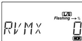
**20. Revolution mixing (RVMX)** uses the tail rotor to suppress the torque reaction of the main rotor due to changes in collective pitch. It is disabled whenever Idle-Up or Throttle Hold are activated.
