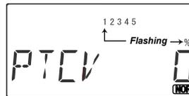
Like the throttle curve described above, pitch curves are tied to the position of the collective stick, and are specified at five points labeled 1 through 5 below. Setup
