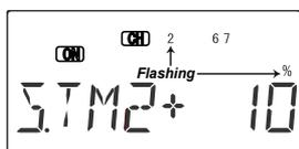
**30.** (4WNG only) You may also set up the speed mode presets (S.TM2) for high speed cruise between thermals. Reflex the entire trailing edge a very small amount -10% or even less all the way across is recommended for starters. The trailing
