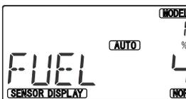
you can check the fuel amount of your model using HTS-SS with HTS-FUEL, fuel level can be checked by appears numeral 0 to 4.(this function only can use HTS-SS. HTS-SS BLUE cannot provide this function)
