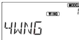
with two ailerons and two flaps. Press the Up arrow until you see the word "WING" in the upper right of the display. The wing type in the lower left will be flashing.
