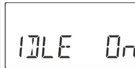
The IDLE ON warning is displayed when the transmitter is powered up with the Idle-up switch on in the helicopter mode only.
