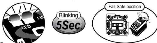
**5** BLUE LED will glow steady once the setting process is completed during above 8sec.
