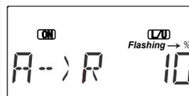
**31.** If desired, add aileron rudder coupling (A->R) for coordinated turns. This setting is highly dependent on the model configuration.
