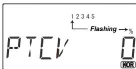
**19. Pitch Curve.** You can use the Pitch Curve (PTCV) menu's five-point setting curves to make finer adjustments
