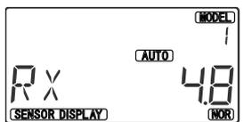
Pressing the Down button gives the Telemetry information display when you use Optima series receivers(Hitec Telemetry capable receivers) you can check receiver voltage
