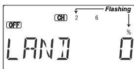
1. Use the Edit Up Down arrow keys to select the LAND window. Depending on the position of the landing switch, the display will show OFF or ON. The Flt. Mode switch turns on LAND when all the way forward.
