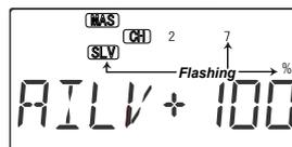
7. Press the Cursor Right key once, Highlighted SLV sign and numeral 7 will be flashing that representing right elevator moving direction. Move the elevator stick all the way to the back
