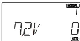
This screen appears at startup. The model memory number is shown by state in figures. Battery voltage is shown in the bottom left, and operating
