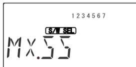
1. To set the MX.SS, get to the MX.SS screen with the Edit Up Down keys (press at the same time, and then search MX.SS by pressing Edit Up or Down repeatedly). In the display has
