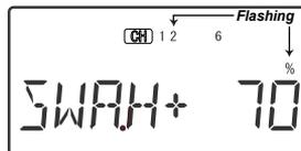
7. If all the servos tilt the swash aft with up elevator stick, go to the next step. If they tilt the swash forwards, press the Cursor Right key once to get to the elevator setting menu
