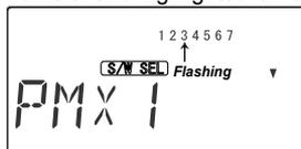
3. You can be assigned new mixing channel by pressing Data +Increase, -Decrease keys or toggle switch. also you can check the new assigned switch which being set (by numeral flashing) or On or Off status..
