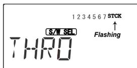
5. Pressing the Cursor Right to find THRO function. This is only can use in Glider type. Current 3CH function (Motor On/Off or Spoiler) can be assigned by throttle Stick or other switches.
