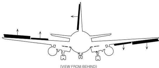
Aileron->Flap mixing is turned on and off with the Flt. condition switch. You can adjust the amounts of up and down mixing independently, which is nice if your model's flaps are hinged on the bottom and they cannot move up past a certain point.
