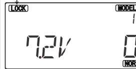
Pressing the Lock button locks the throttle servo and holds it where you last commanded it. This may be used as a safety feature when you are carrying the model and transmitter to
