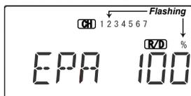
**39.** To set the UP elevator motion, press on the Right Cursor key until the channel 2 will flashing. Now move the right stick all the way to the transmitter bottom and hold it.
