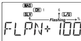
7. Now you'll input the amount of flap response on the flaperons. The flap motion is commanded by the VR1 knob to the left back of transmitter, and both flaperons should move the same direction when you move the knob. Press the Cursor Right key one time, so the Numeral 6 and MAS will be flashing that indicating flaps are now the master channel, indicating left (CH6) flaperon.
