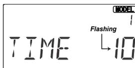
**9. Set the stopwatch.** Press the UP arrow four times. This gets you into the Timer menu (TIME). Use the Data Increase and Decrease keys to select the amount of time you want the stopwatch to count down. This is handy to keep track of engine running time so you don't run out of gas.
