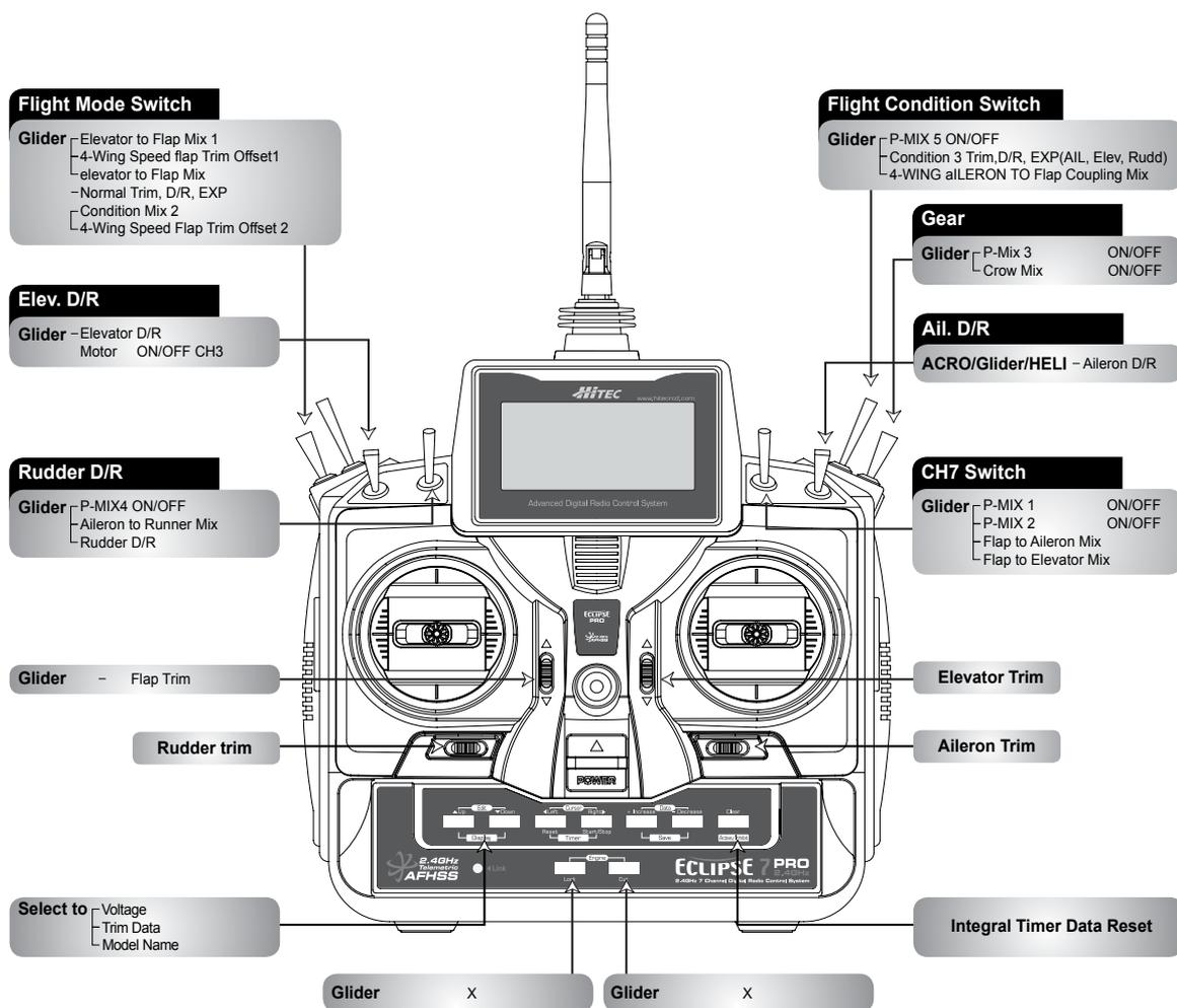
This figure shows the assignments for a Mode 2 system as supplied by the factory for the North American version. Note that some of the functions will not operate until activated in the mixing menus.
