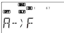
14. (4WNG only) Move to A ->F by pressing the Up Down Edit buttons. Activate it by pressing the Active/Inhibit (Clear) key ('On' or 'Off' will be flashing
