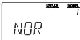
**4. Swash Type.** Now it's time to select the swash type. Select NOR for helis with independent aileron, elevator, and pitch servos; 120' for models using 120 swashplates;
