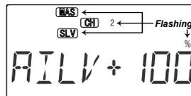
6. Press the Cursor Right keyonce. Highlighted MAS, SLV sign and numeral 2 will be flashing that representing left elevator direction, and the percent indicator will blink on and off.
