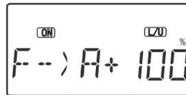
1. Locate the flap->aileron mixing function by scrolling to the F->A menu with the Up Down Edit keys. The default is for it to be inhibited (Inh). Press the Active/Inhibit
