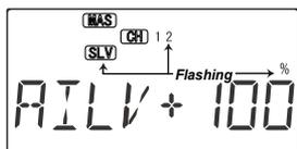
4. Press the Cursor Right key once. Highlighted SLV sign and numeral 2 will be flashing that representing left elevator slave channel, and the percent indicator will blink on and off.
