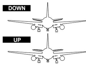
**20.** If the elevator control moves in the wrong direction, move over to Channel 2 by pressing the Cursor Right key. Now the '2' should be flashing in the display. Activate the opposite direction for the elevator servo by pressing the Active/Inhibit (Clear) key. Move the right-hand stick up-and-down again and verify the elevator moves the right direction.
