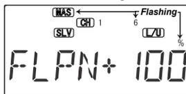
6. If the left (CH6) flaperon moves correctly with aileron stick, go to the next step. If not, please check again above 4 and 5 steps.
