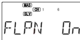
3. Press the Active/Inhibit (Clear) key to activate the flaperon function. This will show the On indicator.
