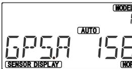
You can check the Altitude of your aircraft using HTS-SS BLUE, HTS-SS with HTS-GPS. GPS Altitude value appears in lower right in the display. GPS Altitude range is 0 to 999m
