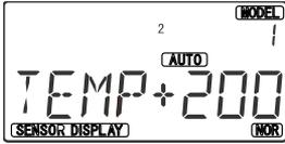
As you see to left diagram, this information coming from HTS-SS BLUE ,HTS-SS temperature sensor second slot. You can see small numeral 2 in the display This is showing
