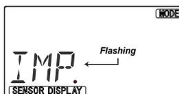
1. With the transmitter switched off, turn on your transmitter while pressing both of the two Edit keys (the two keys on the far left). The Imperial select (IMP) menu will be displayed .
