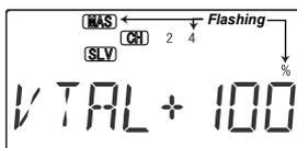
6. Now you'll input the amount of rudder stick response on the left (CH4) ruddervator by pressing the Cursor Right key once. Now the numeral 4 and MAS will be flashing, and you may
