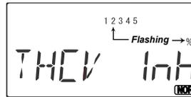
4. When you're finished with Point 1, move to the next point with the Cursor Right key. The numeral 2 should be flashing that indicates you are setting the value for
