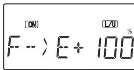
1. Get to the flap->elevator mixing function by locating the F->E menu with the Up Down Edit keys. The default is for it to be inhibited (Inh). Press the Active/Inhibit (Clear)
