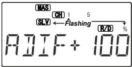
differential on the second aileron. Holding the aileron stick to the left, we leave the percentage setting at 100%. Now move the aileron stick to the right and use the Data -Decrease key to drop it to 70% or so. Now, when you move the aileron stick, each aileron will go up more than down.
