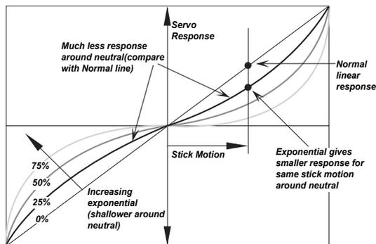
You will notice that exponential has a smooth curve. For this reason it is possible to have low sensitivity at low stick angles (like dual rates), and yet have full motion at full stick deflection. The Eclipse 7 Pro allows you to have
