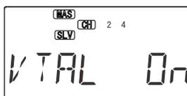
3. Press the Active/Inhibit (Clear) key to activate the V-tail function. The display will show On.
