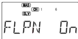
**14.** Turn on the Flaperon function by pressing the Active/Inhibit button (Clear) until "On" appears in the display.
