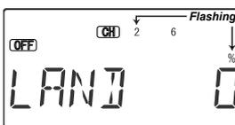
2. First the amount of elevator offset is programmed. The numeral 2 will be flashing (representing elevator). You may adjust the amount of travel with the Data +Increase and Decrease keys.
