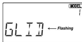
4. Press the Up arrow until the word GLID appears, flashing on and off. If it does, you're ready to proceed on to the next step. If not, press the Left or Right Cursor keys until it
