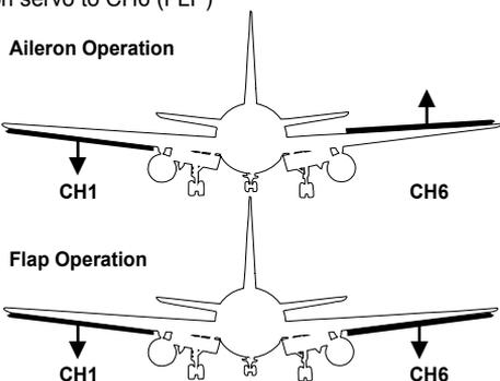
You can combine the flaperon function with the landing function (LAND), to get steeper descents without building up airspeed. This is very convenient for making short approaches on small fields. Note that you cannot have both flaperon and elevon mixing active at the same time.
