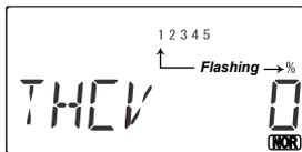
**18. Throttle Curve.** You can use the Throttle Curve (THCV) menu's five-point setting curves to fine-tune the engine servo's response.
