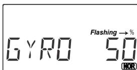
**21. Gyro settings.** You can select an independent value of gyro gain for each flight condition by using the GYRO menu. Select the desired flight condition, then use the Data keys to choose the
