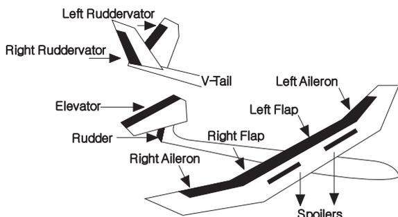
1. Before you begin, be sure that all of your aileron and flap servos are plugged into the proper receiver channels:
