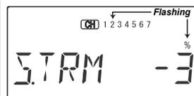
29. Repeat the subtrim adjustment with the elevator servo (CH2). First set the pushrod length mechanically to get as close to neutral as possible, then set the subtrim to
