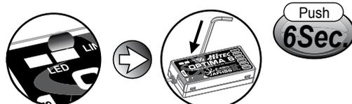
**3** Release the link button when LED is turned off.
