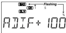
1. Press one of the Up Down Edit buttons repeatedly to select the ADIF window. To begin with, the function is already activated, but it's set to 100% on both sides so there is no differential.
