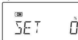
5. If you want to change Set position, press the Cursor Right key to change the position of Flap control channel (VR1) which value you need, and then press Clear key.
