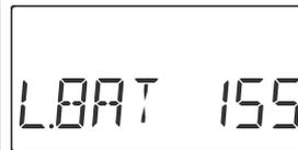
The LOW BATTERY warning is displayed when the transmitter battery voltage drops below 6.6 volts, and a beeper sounds.
