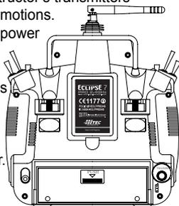
The instructor's transmitter has normal control over the model unless the trainer switch is pulled, passing control to the student's transmitter. If the student loses control, the instructor can quickly "take over" by releasing the trainer switch and controlling the model.
