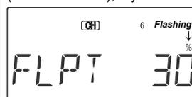
**45.** If you wish to have the flaps operate with the CH6 knob, go back to the FLPT menu and input a number greater than zero. Adjust the number to get the
