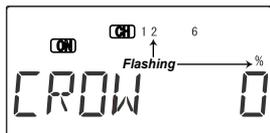
zero or very little elevator compensation until you fly and determine what is needed: if the model pitches up with crow, add down elevator compensation and if it pitches down wards, add some up compensation. Make only small changes in compensation because it has a big effect on trim. Refer to the sailplane trimming chart for more details.
