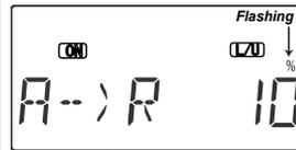
1. Press one of the Up Down Edit buttons until the A->R window appears, as shown. The default is for the function to be inhibited, as shown. To activate, press the Active/Inhibit (Clear) key.
