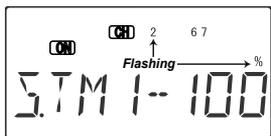
1. Start by locating the S.TM1 menu with the Up Down Edit keys, then pressing the Active/Inhibit (Clear) key. Either the 'Off' or the 'On' display will be flashing, depending on the
