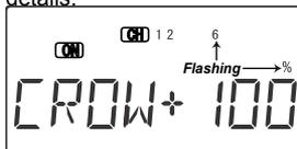
6. Now press the Right key to get to the flap setting menu (the numeral 6 and percentage sign will be flashing in the display). Press the
