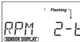
1. With the transmitter switched off, turn on your transmitter while pressing both of the two Edit keys (the two keys on the far left). The RPM select (RPM) menu will be displayed . you can check aircraft RPM using RPM sensor (You can use maximum 2 RPM sensors).
