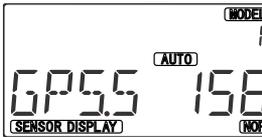
You can check the Speed of your aircraft using HTS-SS BLUE, HTS-SS with HTS-GPS . GPS Speed value appears in lower right in the display . GPS Speed range is 0 to 999 Km/h.
