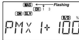
2. Now you'll select the Master channel for the mixing, the channel that causes the mixing to occur. Press the Cursor Right key twice to get the master channel (MAS will be appear), then press the Data +Increase or -Decrease keys to move the number of the desired master channel, 1 - 7.
