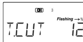
**17. Throttle Cut.** Enter the throttle cut (T.CUT) menu and enter a value of -25% or so. Press the Cut button and be sure that the carburetor fully closes, which will shut off the engine. Don't pick too large a number, or binding may occur.
