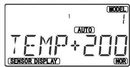
You can check the temperature of your aircraft's engine , muffler , ESC , batteries and etc. that using HTS-SS BLUE, HTS-SS with HTS-TEMP(You can use maximum 4 temperature sensors).
