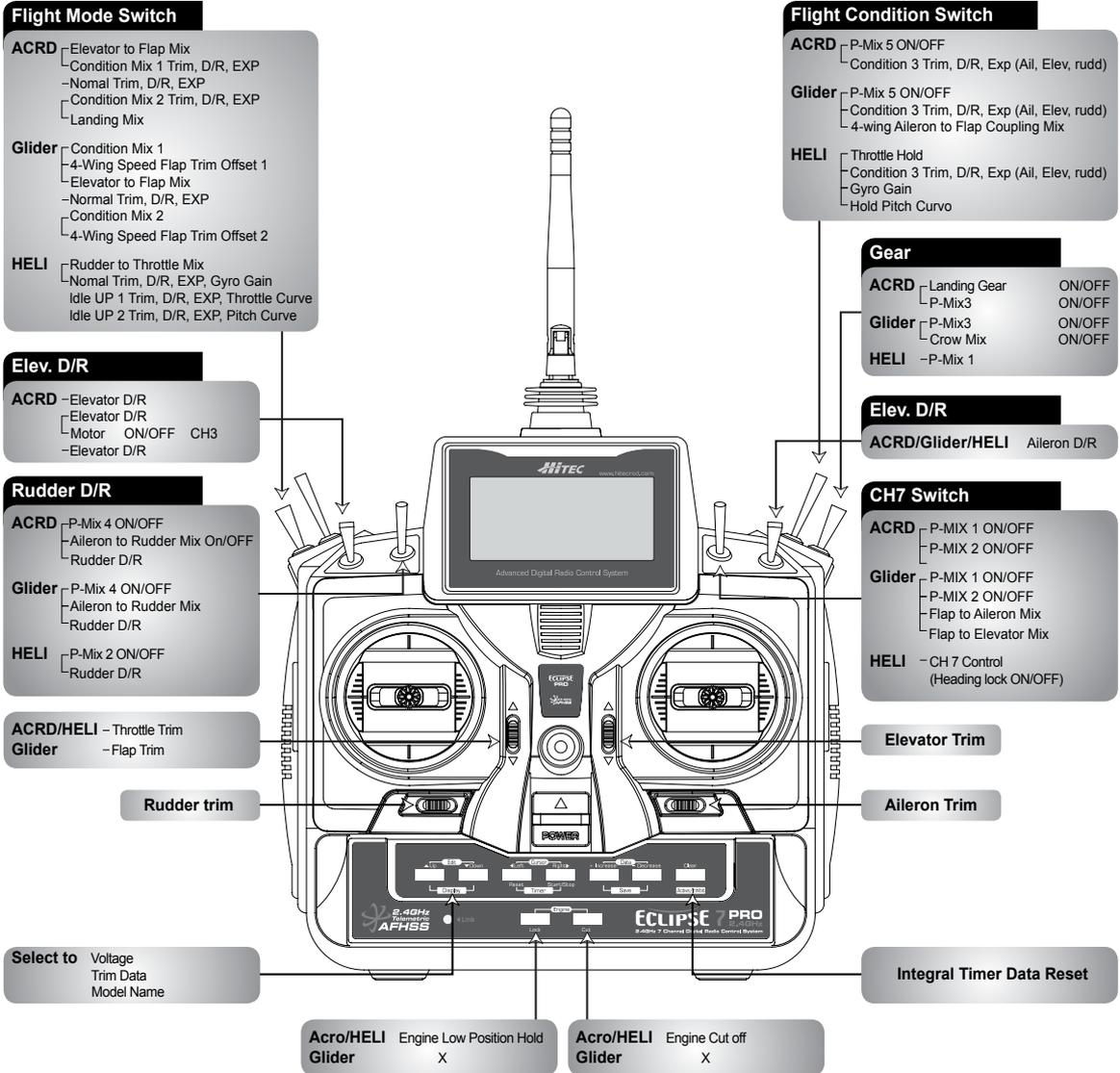
This figure shows the assignments for a Mode 2 system as supplied by the factory in North America. Note that some of the functions will not operate until activated in the mixing menus.
