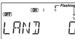
3. To get to the flap travel setting, press the Cursor Right key. The channel numeral 6 will be flashing, indicating the flap channel. You may input any desired
