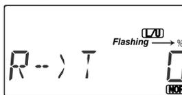
1. Press one of the Up Down Edit buttons repeatedly to select the R->T window. The function is activated by switching the Flt. Mode switch all the way
