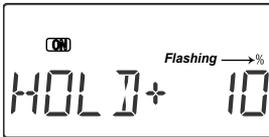
2. Now you can adjust the throttle hold position with the Data +Increase or -Decrease keys, anywhere between -50 and +50% (To inhibit this feature, press the Active/Inhibit (Clear) key).
