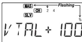
4. Press the Cursor Right key once, to get to the elevator setting menu. Highlighted MAS sign and Numeral 2 will be flashing that representing elevator master channel, indicating the right (CH2) ruddervator, and the percent indicator will blink on and off. Move the elevator stick all the way to the back (full up position): both ruddervators should move upwards. If the right (CH2) ruddervator moves down,
