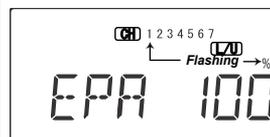
**14. Servo Travel.** Use the EPA command to limit servo travels to prevent binding.
