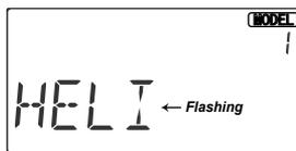
Right Cursor keys until HELI appears. You must press both Data keys to "Save" the setting. This is how you select the type of model you wish to use, either ACRO, HELI, or GLID.
