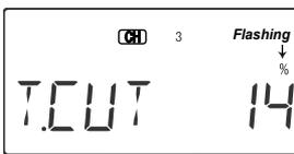
button. A maximum of 72% may be chosen, but only use the amount you need to fully close the carburetor without stalling the servo.
