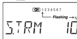
**13. Servo Neutrals.** First, be sure the hovering pitch and hovering throttle knobs are centered. Set up all linkages so that all servos are as close to mechanical neutral as possible. Then, use the Subtrim (STRM) window to make fine adjustments on the servo neutrals.
