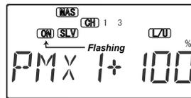
1. Call up the mixer screen by repeatedly pressing one of the Edit Up Down keys until a PMX window appears. The default is for the function to be inhibited. To activate, press the Active/Inhibit (Clear) key. This will cause the INH display to change to a display showing 100%, Master and Slave indicators, and a flashing ON or OFF depending on the position of the mixer's on-off switch.
