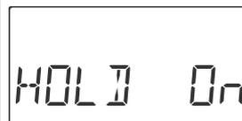
The HOLD ON warning is displayed when the transmitter is powered up with the Throttle hold switch on in the helicopter mode only when throttle hold values are
