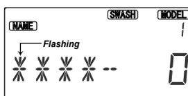
**5. Name your model.** Press the Down arrow once. This gets you into the model name mode (note the words MODEL and NAME in the upper left of the display).
