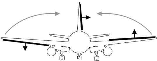
The slower the model flies, the more mixing is needed, and the faster it moves, the less is needed. It is ideal to make slow-flying scale models fly realistically.
