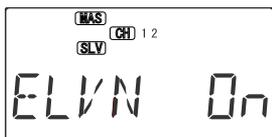
3. To activate, press the Active/Inhibit (Clear) key. The letters "INH" will turn to "On."
