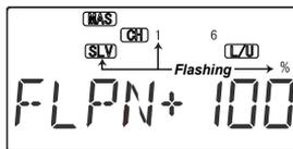
5. Press the Cursor Right key once. Highlighted SLV sign and numeral 1 will be flashing that representing right aileron slave channel, and the percent indicator will blink on and off.
