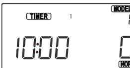
Pressing the two Timer button at the same time that gives the Timer display .you can start the timer pressing Start button . Stop and Reset also same function as like key name.
