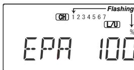
**1.** Enter the programming mode by pressing the two Edit Up Down keys (the two keys on the far left) at the same time. You should pop right into the EPA screen,
