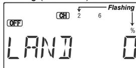
**59.** Press one of the Up Down Edit buttons until the LAND window appears, as shown. The landing mode is OFF unless the Flt. Mode switch is fully forward.
