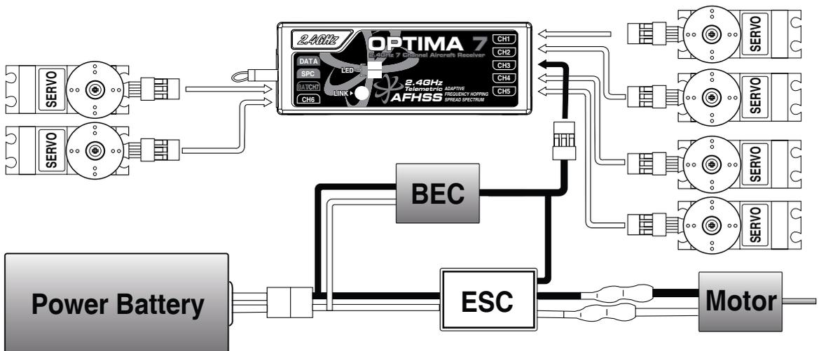
Optional BEC shown in diagram is used if the servo power requirements exceed that which the ESC provides.
