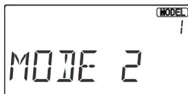
1. With the transmitter switched off, turn on your transmitter while pressing both of the two Edit keys (the two keys on the far left). The Mode select (MODE) menu will be displayed . You can change the Mode 2 to Mode 1, Mode 2 to Mode 3 or 4.
