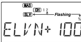
8. Move the elevator stick all the way to the back (full up position): both elevons should move upwards like elevators. If the left (CH2) elevon moves down, change its
