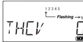
3. You begin at set point #1, idle. Numeral 1 should be flashing in the display, and a value of 0% should be shown. Press the Data +Increase or -Decrease key to change the setting to your desired value.
