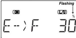
1. Press one of the Up Down Edit buttons until the E->F window appears. The default is for the function to be inhibited. To activate, press the Active/
