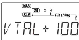
7. Now you'll input the amount of rudder stick response on the right (CH2) ruddervator by pressing the Cursor Right key once. Now the numeral 4 SLV will be flashing,
