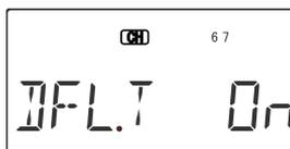
1. Turn on Dual Flap Trim by locating the DFL.T menu with the Up Down Edit keys. The default is for it to be on. If you wish to disable the dual flap trim, press the Active/Inhibit (Clear)
