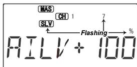
5. Press the Cursor Right key once. Highlighted SLV sign and numeral 7 will be flashing that representing right elevator slave channel, and the percent indicator will blink on and off.
