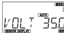
BLUE with HTS-VOLT which attached receiver or Electric powered aircraft's main battery. Voltage value appears in lower right in the display as you see left diagram . voltage range
